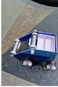
Figure 8: Shallow-water trial of prototype AquaTrace, confirming hull buoyancy, paddle-wheel propulsion, and filtration module stability under wet operational conditions
