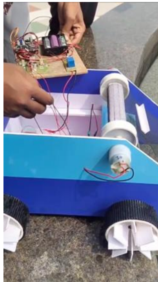
Figure 7: Bench-level proof-of-concept prototype showing the stage 1 coarse mesh filter, motor assembly, and initial electronics stack
